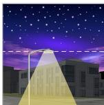
The Upward Light Ratio (ULR) and Upward Light Output Ratio (ULOR), the latter taking the flux from the luminaire into account, provide information on the percentage of light emitted towards the sky. This Schréder range of luminaires minimises or eliminates (depending on the options) upward-directed light flux. It complies with strict international and local requirements.
