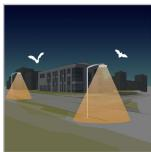
If not well designed, artificial lighting can badly affect wildlife. Blue light and excessive intensity can have a damaging effect on all types of life. Blue light radiation has the ability to suppress the production of melatonin, the hormone that contributes to the regulation of the circadian rhythm. It can also alter the behavioural patterns of animals including bats and moths, as it can change their movements towards or away from light sources. Schréder
