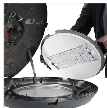
FLEXIA QUERCUS includes an instant electrical disconnection on opening and a complete tool-free removable LED engine.
