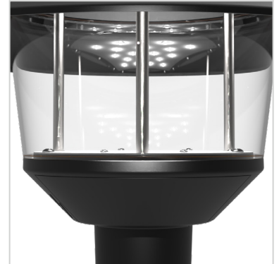
The body assembly is pressure die-cast aluminium with stainless steel fixings and the radial visor is injection moulded acrylic
