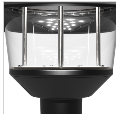
The body assembly is pressure die-cast aluminium with stainless steel fixings and the radial visor is injection moulded acrylic
